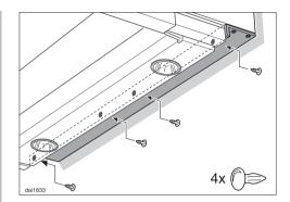
Connect the space bar from the rear with 4 plastic rivets at the hood rear side.
